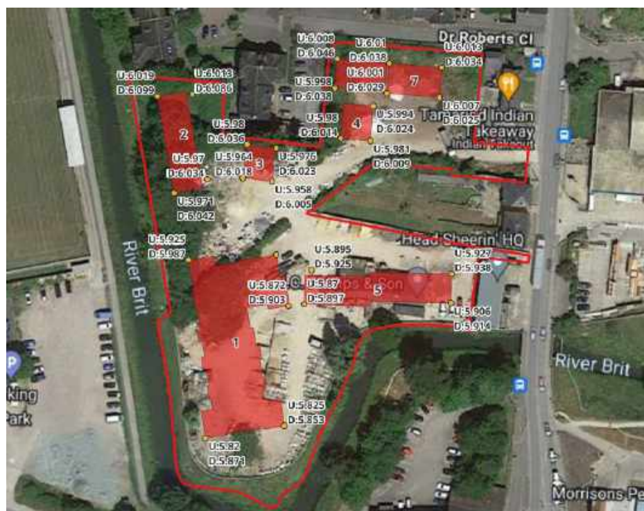
Figure 3.1 – Design flood levels at proposed buildings
