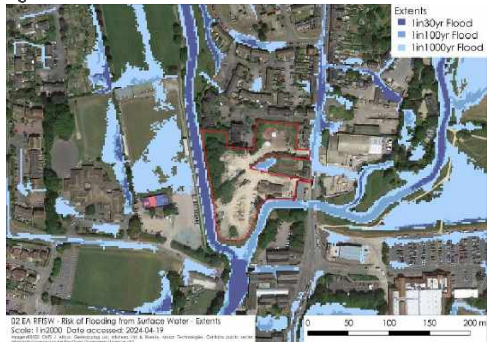
Figure 2.5 – Flood Risk from Surface Water
